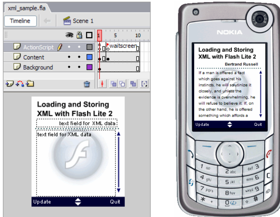
Figure 11 Screens of a Flash Lite authoring environment and the result of its execution shown by an emulator.
